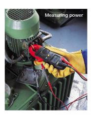
With its W position, the F05 clamp transforms itself into a wattmeter and measures both the active power and the power factor in single-phase systems. The immediate mode indicates the phase order in a three-phase system. With the original "2-wire" method (Pfisterer license), it's quick and practical.
