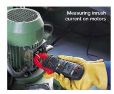
When starting, certain loads (like those of motors), heating resistors and lighting systems require a strong rush of current which can trigger the safety system and even damage the installation.
