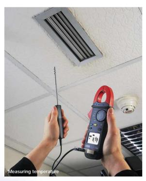
By adding a simple sensor, the Temperature function on the F03 and F07 clamps measures surface and ambient temperatures in °C or °F.
